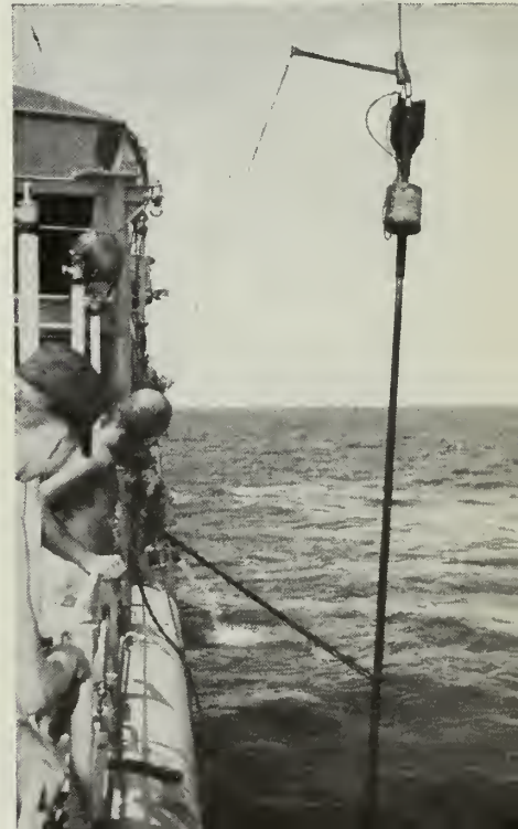
MUDDY MEASURE —Mud brought up by corer is checked. Below: Ewing corer is set for drop into ocean's floor.
